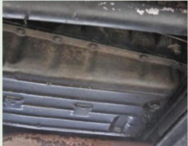
*An angle finder can be placed on the transmission pan or any other machined flat surface of the engine, tranny, diff or transfer case that's parallel or perpendicular to the centerline.*
