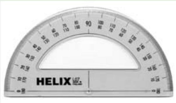
*Add a string and plumb bob to an inexpensive protractor and you have a perfectly suitable tool for measuring driveshaft slope.*
