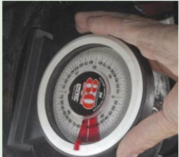
*Tom Wood prefers to measure pinion slope by placing the angle finder on this machined portion of the axle housing. Several angle finders, ranging from dirt cheap to quite pricey, will do the job.*
