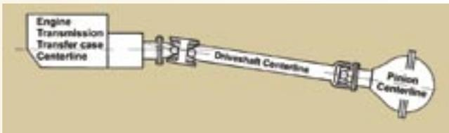
*This illustration shows the proper geometry for a driveshaft featuring a double cardan joint and conventional U-joint.*
